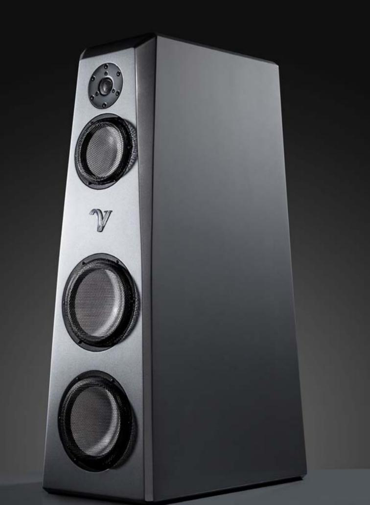
Fabricated using VSA's patent-pending Triple-Wall Laminate Construction, my review pair's enclosures were finished in an impeccable piano-black lacquer. The outermost layer of this composite is a sheet of resin-based MDF (medium density fiberboard). The middle layer is a sheet of synthetic stone—made from crushed gravel, various other minerals, and a resin binder—that's bonded to the inner surface of the MDF outer shell. The innermost layer is hard felt.
